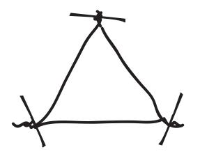
Use three separate wires. Floral wire from Walmart works well. Use three separate people at each corner of the triangle. Each person inserts a rod into one twisted end of the triangle. Each person twists in turn as per the jig instructions until the twists reach the center Then insert a brass tube in the hole and continued twisting will trap the tube. Finishing is the same as for wickholder made with the jig.
